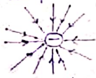
Electric field due to -ve charge.
